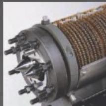
Specially designed barrel heating cooling elements (air power cooling) and precise locations of thermocouples ensures accurate temperature control. The large surface area of cooling elements results into the highest efficiency and lowest maintenance.
