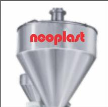
Metering unit facilitates accurate adjustment of the screw feeding factor and plasticizing capacity. It is ideal for materials with the possibility of density variations & particularly suitable for processing regrind and pellets.
